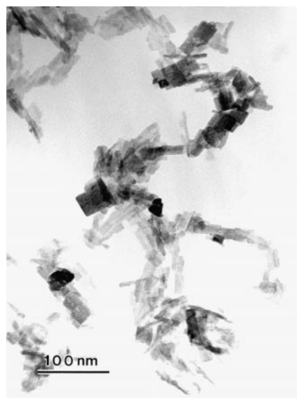
Fig. 7 TEM image of a BZT powder produced with B/M=1 and M=1\text{ mol l}^{-1} .
